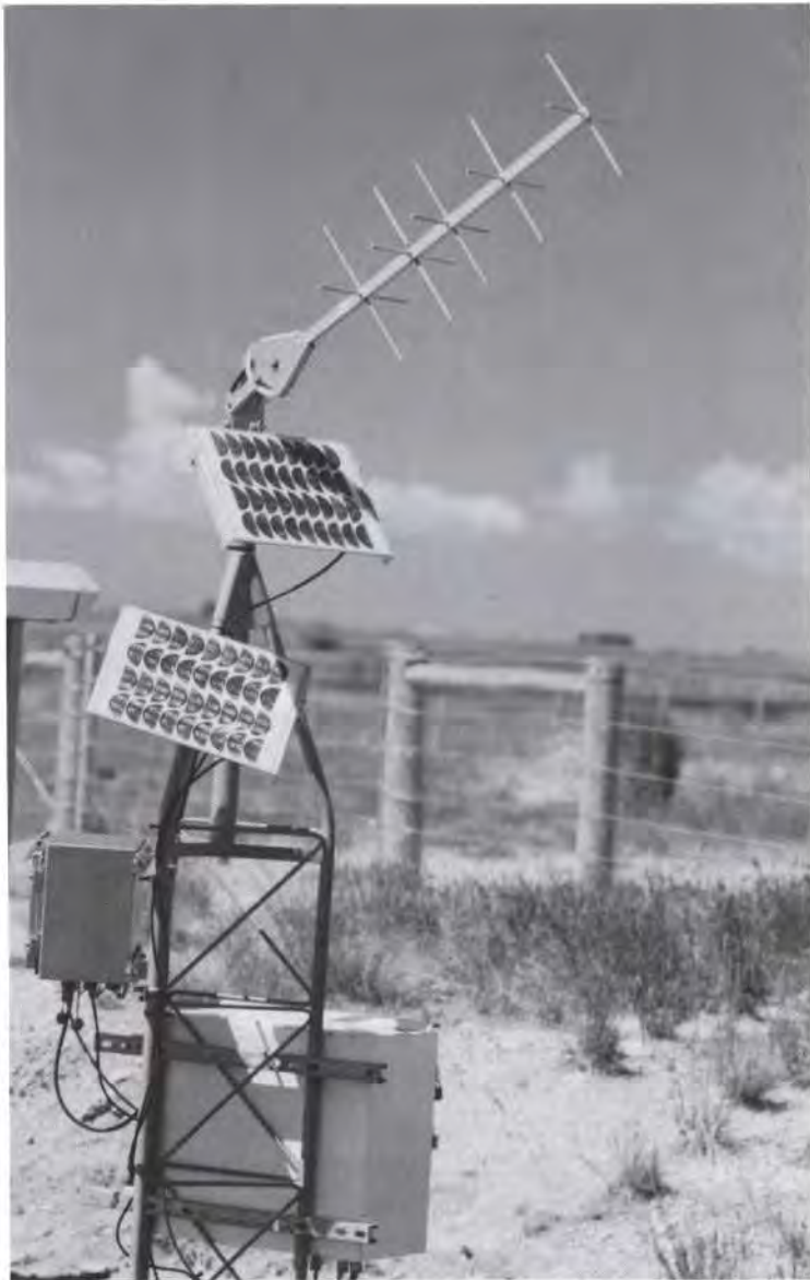
Mid-size PV systems (from a few watts to a few thousand watts) provide power for remote applications all over the world, including water pumping, refrigeration, highway lighting, and village power. Above, photovoltaics power a water-level-monitoring station on the Laramie River in Central Wyoming.
